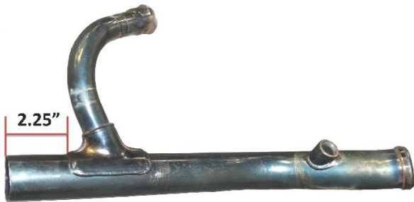
Figure 14 (Header Pipe After Cut / Low Rider, Super Glide, and Street Bob Only)
