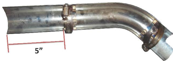
Figure 15 (Chrome Cover After Cut / Low Rider, Super Glide, and Street Bob Only)
